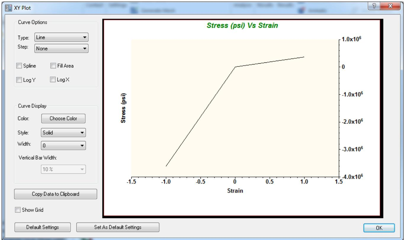
Figure 8. Stress vs. Strain Concrete Function
