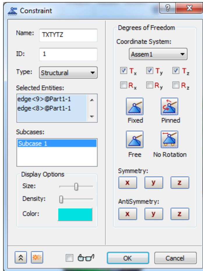
Figure 16. Fix Translations constraint 1 definition
