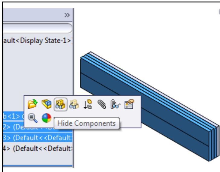
Figure 11. Hide parts in Model tree
