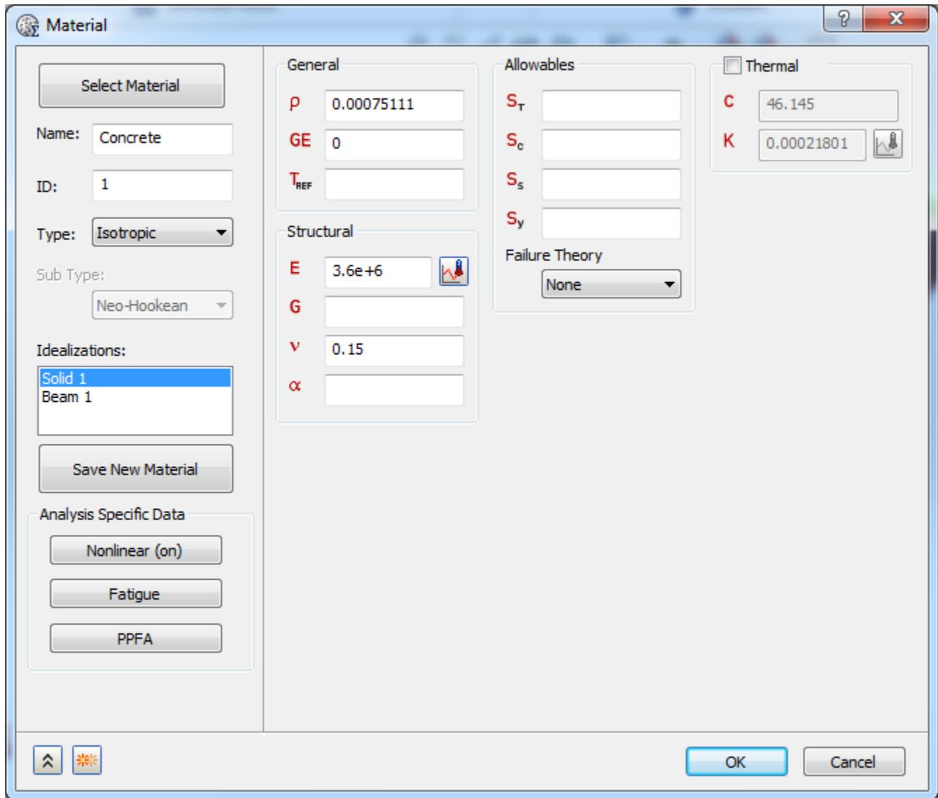
Figure 6. Isotropic Material definition
