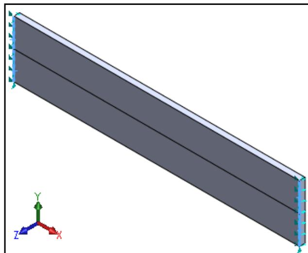
Figure 17. Edges selected for constraint 1 definition
