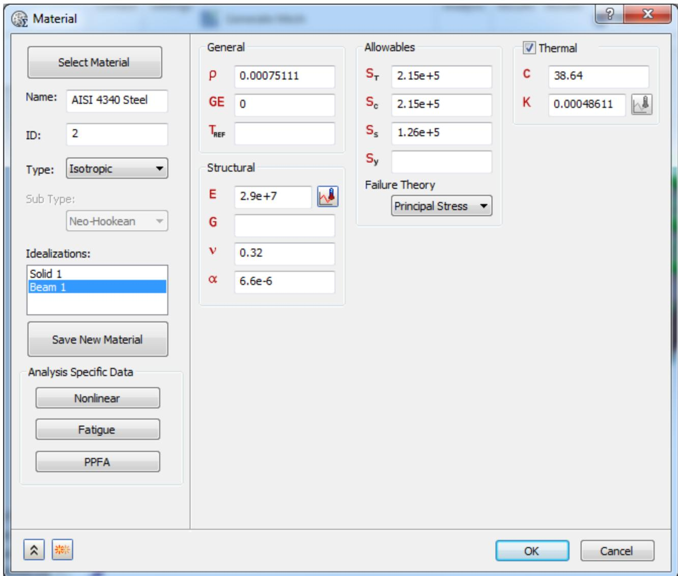
Figure 9. Isotropic Material Definition
