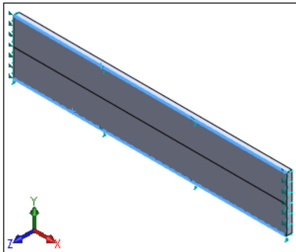
Figure 19. Edges selected for constraint 2 definition
