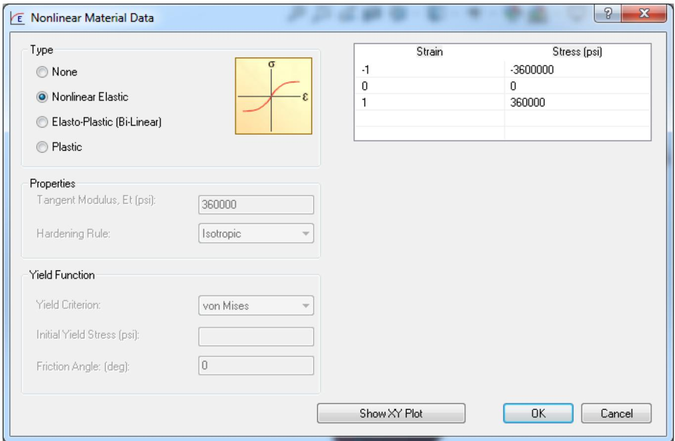
**Figure 7. Nonlinear material settings for the concrete**
