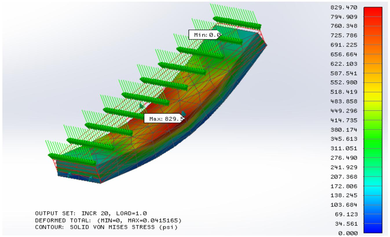
Figure 25. Solid von Mises Stress and Total Translation results
