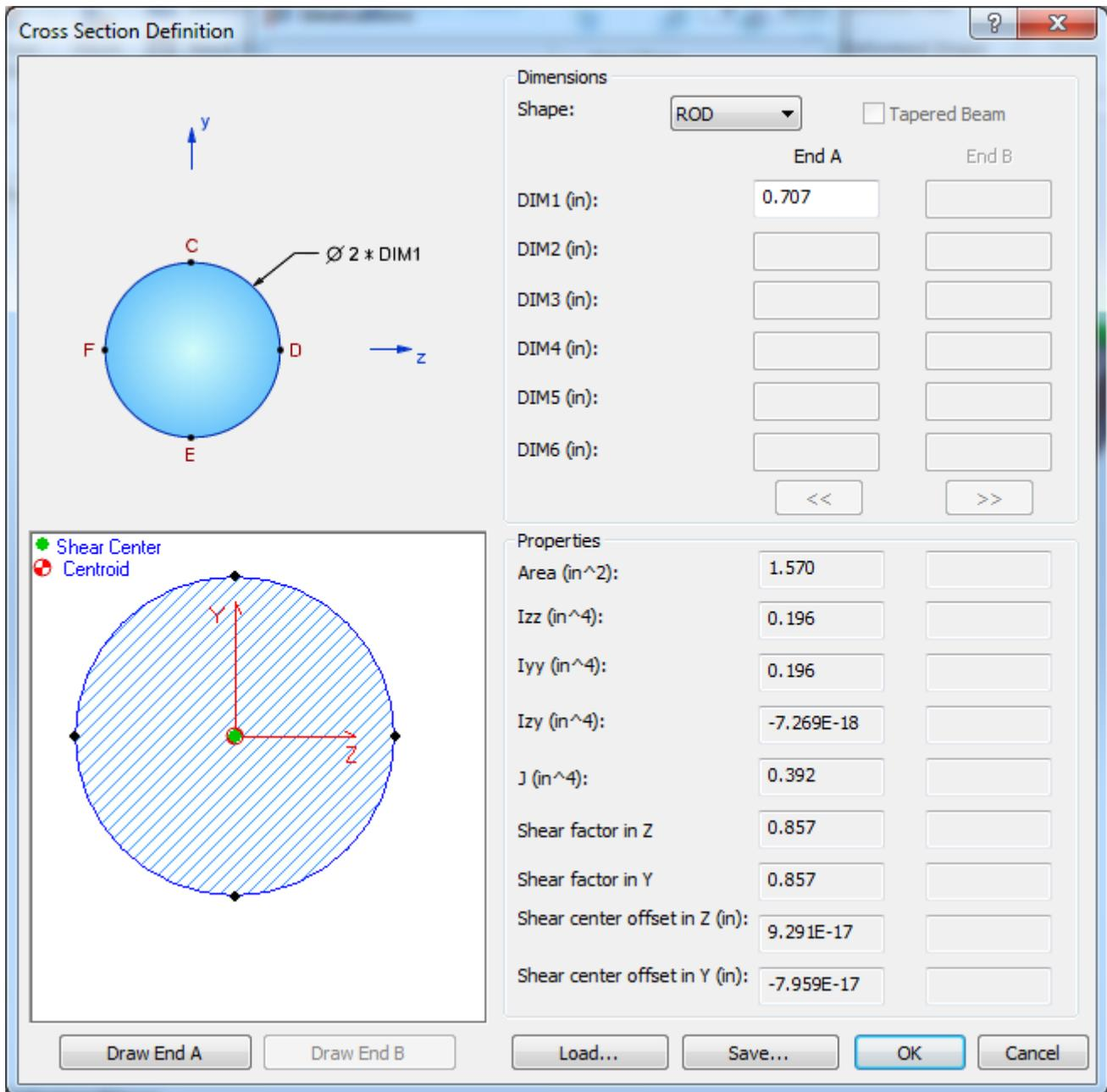
Figure 14. Rod cross section definition
