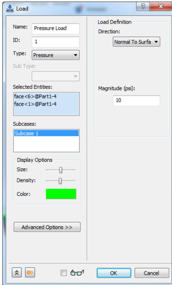
Figure 20. Pressure load definition
