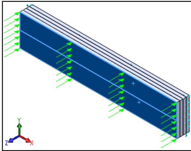
Figure 21. Face selection for pressure load definition
