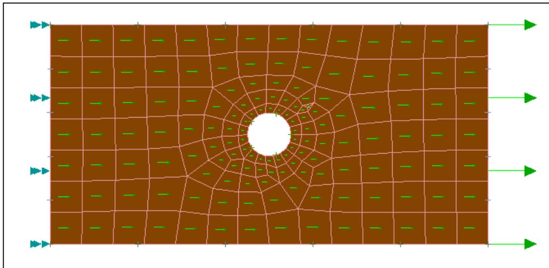
Figure 6. Normal X-Stress with Basic Element/Material Directions
