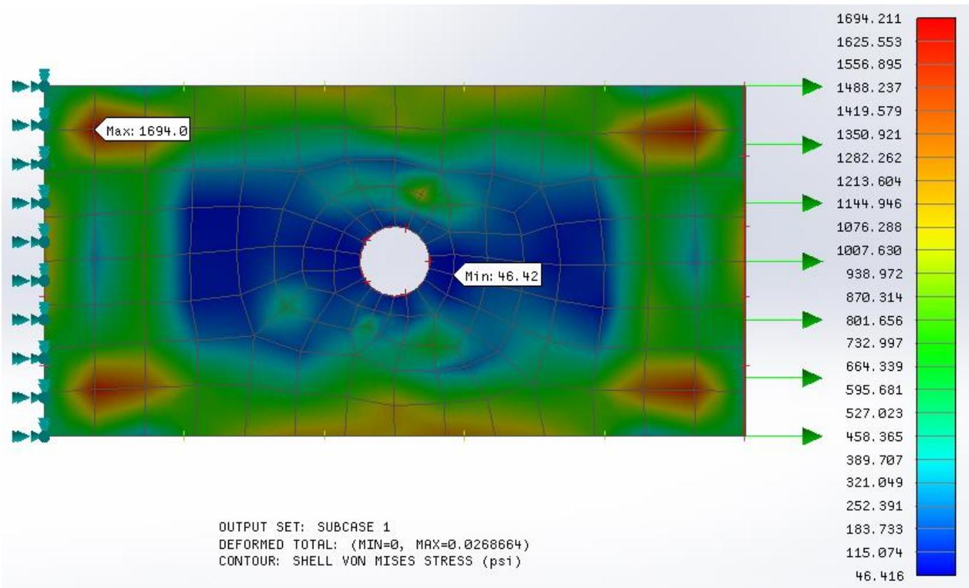
Figure 5. VonMises Stresses with Basic Element/Material Directions.
