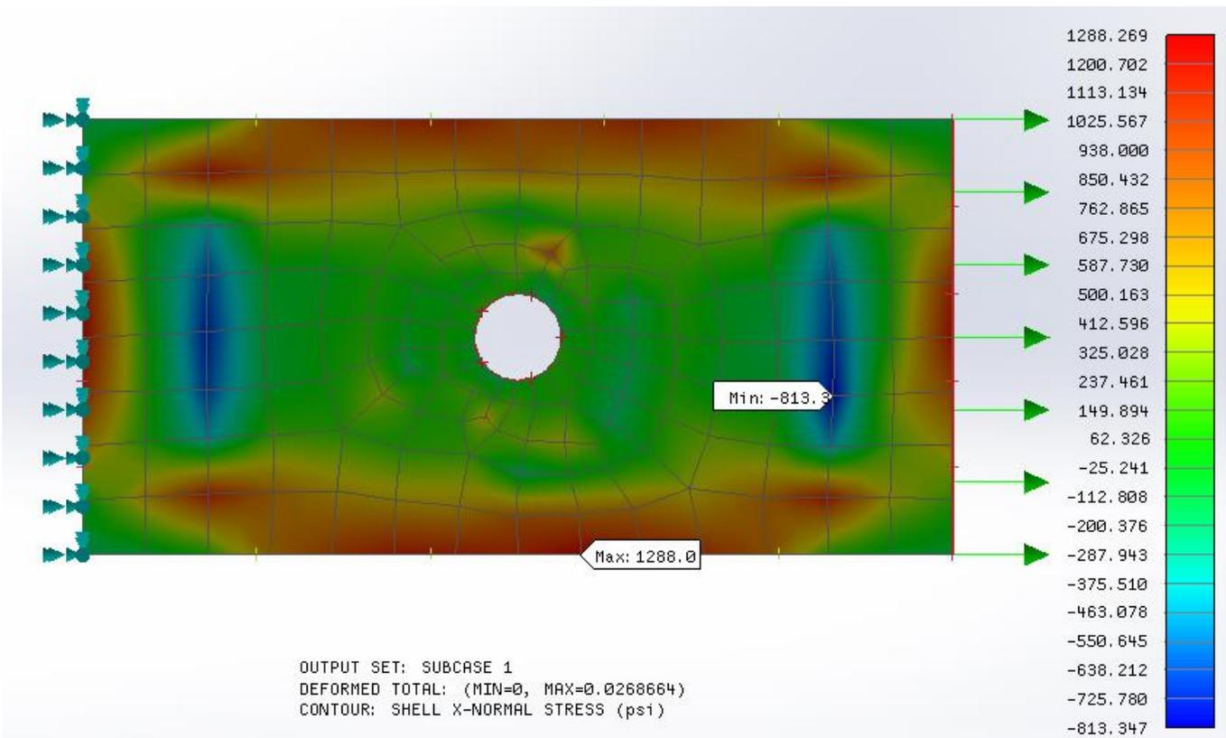
Figure 6. Normal X-Stress with Basic Element/Material Directions.
