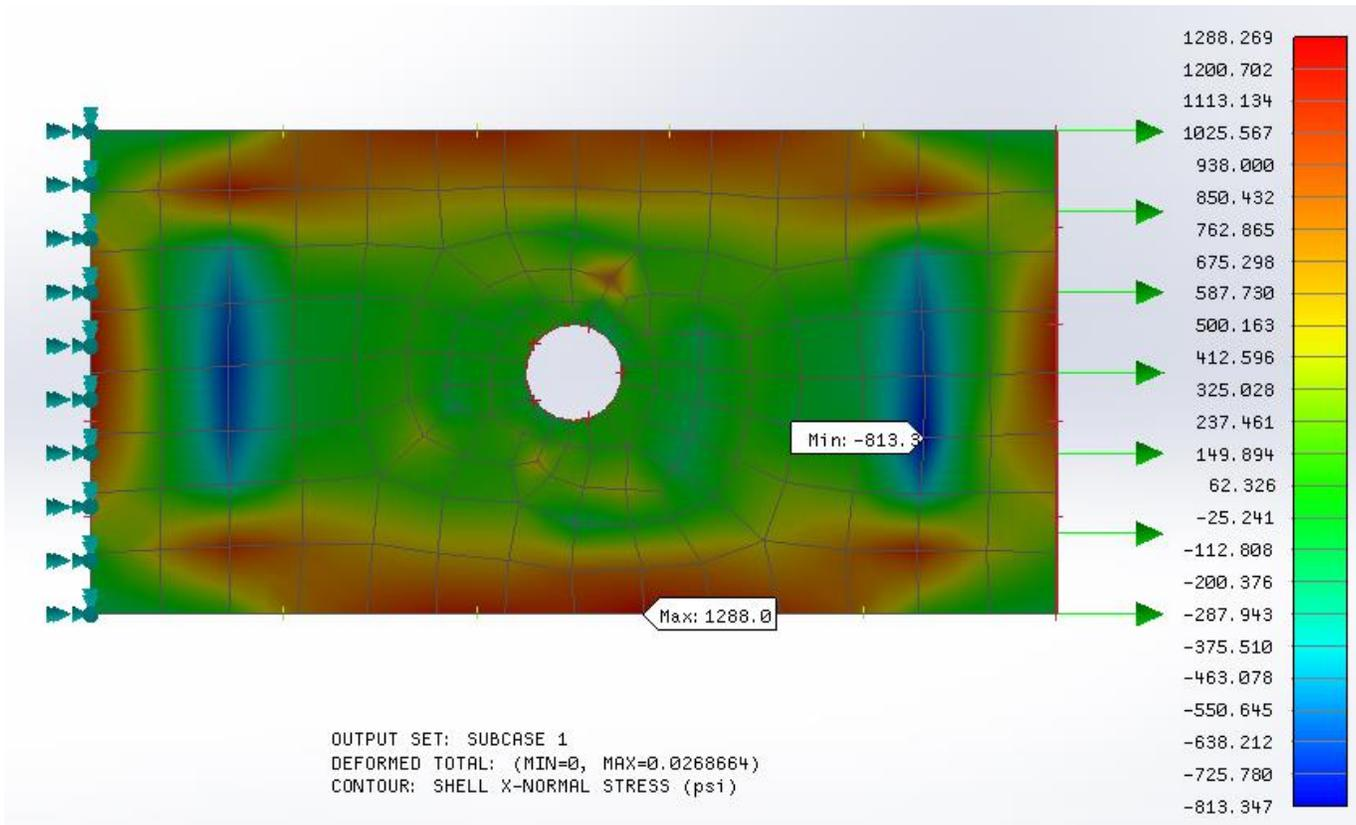
Figure 7. von Mises Stresses after Material Angle Update
